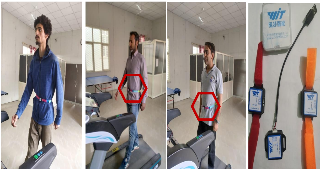
Fig.2 Three different subjects with IMU placed on Umbilical region (centre of mass of the human body) and IMU sensor
